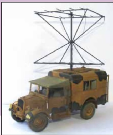
Truck, 15 cwt, 4x2, Wireless (House Type) Mk.III with Radar Light Warning, Fordson WOT2H
